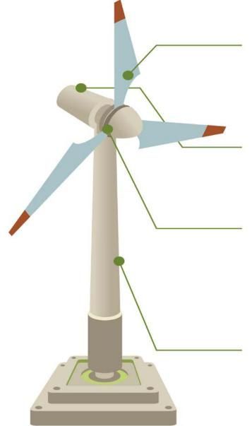
**Blades** – the elements of wind generator, which form the rotor and actuate the main axle by air flow
